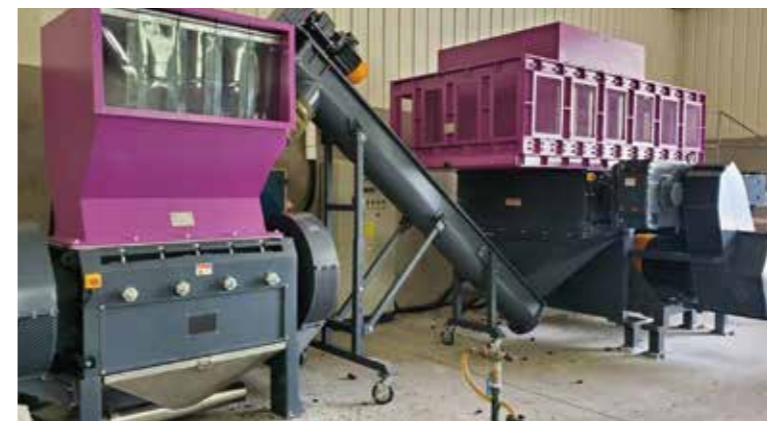
塑料简易破碎线 Plastic Crushing Recycling Line
